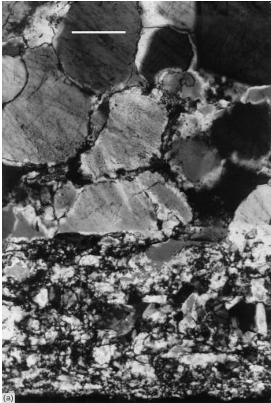
Fig. 6. (a) Photomicrograph of the fault surface (bottom), cataclasite zone (fine grained material just adjacent to fault surface) and process zone (microfractured quartz grains above cataclasite). The scale bar is 0.5 mm in length. (b) Photograph showing the bifurcation of a fault plane around a lozenge of more resistant material. The pen is parallel to the slip direction. The scale bar is 10 cm in length.
